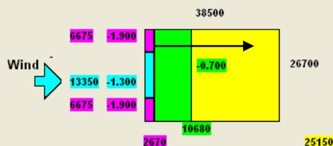
So:  $-1.9 \text{ kN/m}^2$  is critical suction see fixing check
