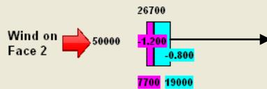
So:  $-1.2 \text{ kN/m}^2$  is critical suction see fixing check
